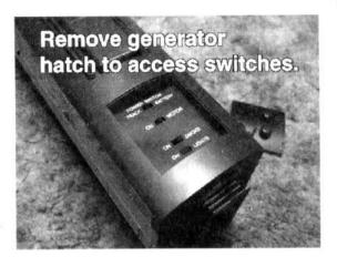
With the front of the locomotive facing away from you, the first or top switch selects track or battery power. In the right hand position the locomotive will run on battery power, in the left hand position, the locomotive will run only on track power.
